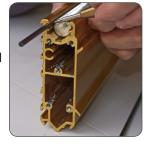
6. Pull on the Red Micro Adjust Knob to snap the Lead Screw Assembly out of the carriage. Again, keep the carriage horizontal when removing the lead screw in order to retain the 5/16" diam-
