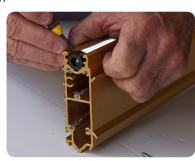
**5.** Use an x-acto knife or a scratch awl to slide the (2) long black plastic rods located on either side of the lead screw out of the carriage.
