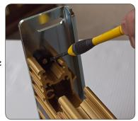
8. Carefully lower the new Lead Screw Assembly into the carriage starting at the forward (fence mounting bracket) end and snap the assembly into position.
