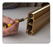
**11.** Re-attach the carriage end plate using the (5) Phillips head screws. TO AVOID STRIPPING THE THREADS, DO NOT USE A POWER DRIVER DURING ASSEMBLY.
