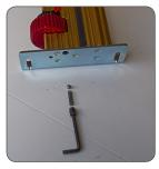
3. Remove locking nut and set screw along with all (5) Phillips head screws from end plate located at rear end of carriage. Remove end plate. Keep carriage horizontal
