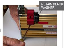
eter ball bearing located inside of the black spacer at the forward end of the lead screw. If necessary, use a screwdriver between the between the carriage and the red knob to GENTLY leverage the lead screw assembly up and out of the carriage. Slide the large black washer located next to the black micro adjust disc off and add it to the new Lead Screw Assembly.
