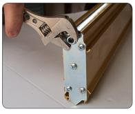
when removing end plate to avoid losing the ball bearing located inside of the black spacer at the rear end of the lead screw.
