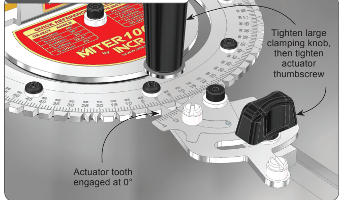
Fig. 8 Square Fence to Blade
