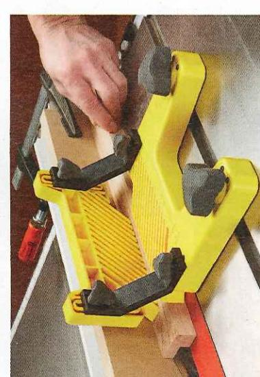
below, anywhere on a cast-iron table. Twist a pair of knobs to engage the magnets and lock the featherboard in place, or twist them again to release it. A vertical attachment kit adds a second featherboard, spacers, and brackets that provide a variety of work-holding options. Extend the top featherboard to apply pressure above the blade, but not against it (above), or mount the second featherboard to press downward while the lower one holds the workpiece against the fence (left).
