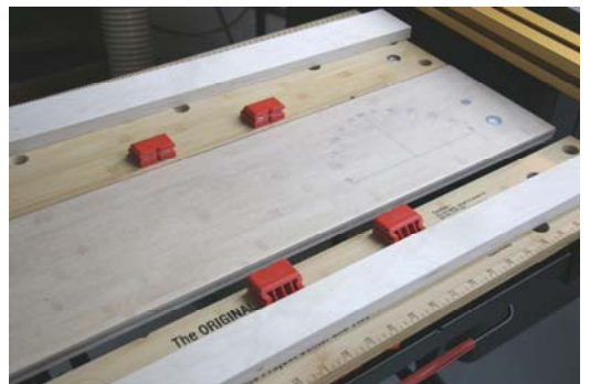
13. A Workmate 425 can form a channel that will align the strips.
