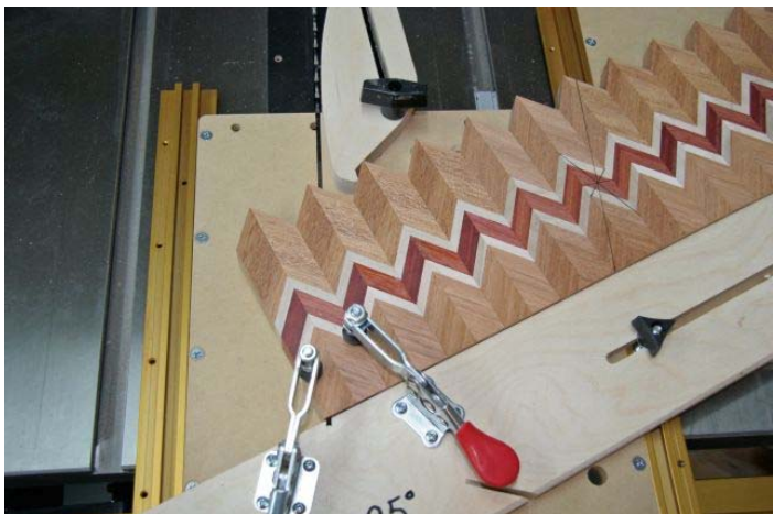
20. Lift the board and reposition it so that the first cut can be made. Save this cutoff for use in the next step.
