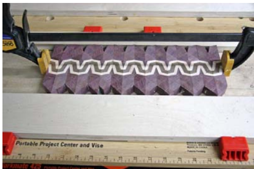
24. Use the channel clamp to align the patterns before clamping from the ends of the board.
