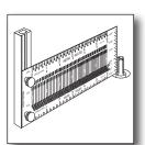
Adjusting the T-Bar: Your INCRA T-Rule comes fully assembled. If you ever loosen the two thumb screws, be sure to place the end of the T-Rule firmly against the indexing lip on the T-Bar before retightening to insure perfect accuracy.
