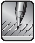
To mark with a 0.5mm Mechanical Pencil: Just hold the pencil vertically and draw a short line in one of the slots, or twist the pencil in a hole to mark a dot.
