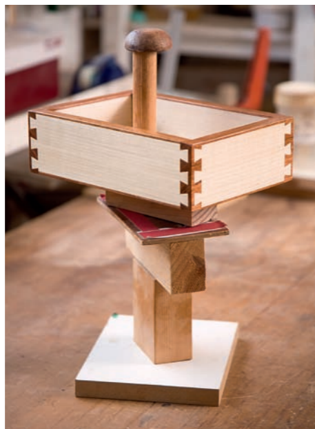
▲ ...and has devised this twisting contraption to rotate boxes by 'remote control' when polishing!
