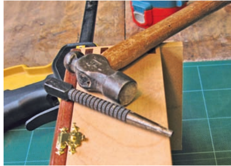
▲ Pic.14 1mm holes were predrilled into the front and the clasp was attached with pins
