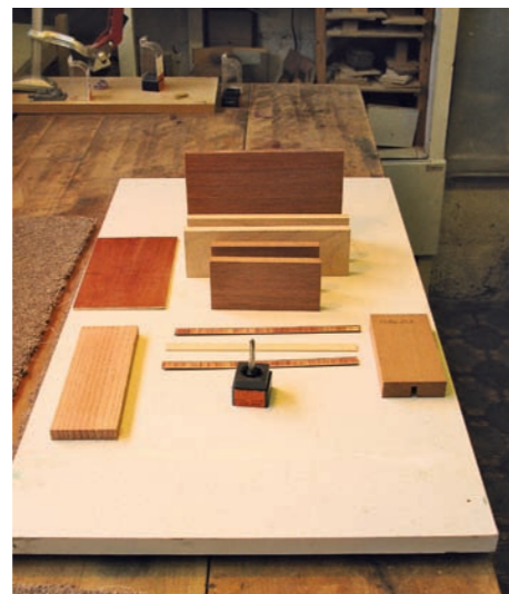
▲ Pic.1 Here are the materials you need for Kieran's box – sapele, sycamore, tulipwood/ sycamore banding, off-cuts, and 1/2in cutter
