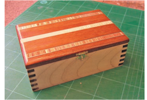
▲ Pic.15 Kieran finished by applying many layers of French polish. You could also use varnish
