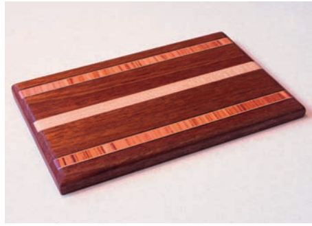
▲ Pic.11 Once dry, lightly sand down the lid with 400-grit paper
