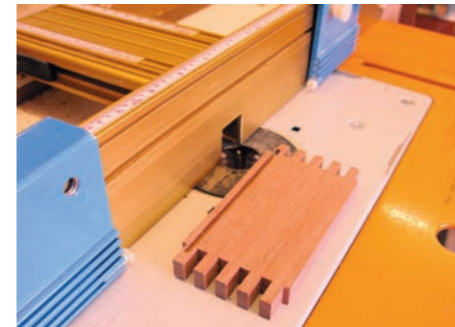
▲ Pic.5 The grooves in the side pieces are stopped grooves to avoid cutting through the fingers
