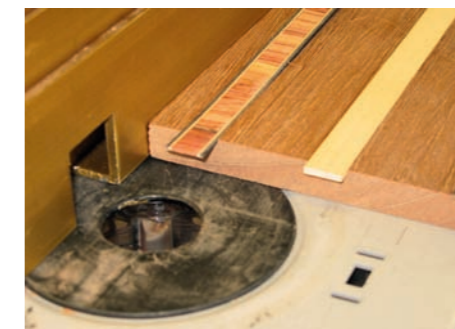
▲ Pic.8 Next, onto the lid – you'll need to cut grooves in it for the sycamore/tulipwood banding
