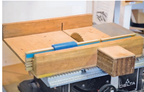
▲ A purpose-built jig enables Incra crosscutting
