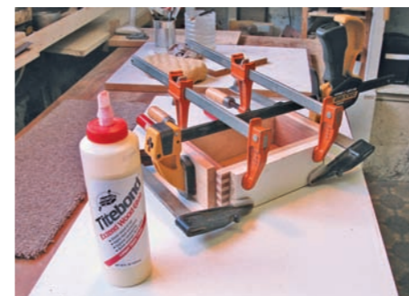
▲ Pic.7 Clamp it all together until the glue has dried. Remove excess glue
