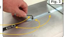
**3** Remove the large clamping knob and disengage the indexing tooth from the protractor. Pivot the protractor head to access and adjust the fourth expansion point. See **Figure 3**. Replace the large clamping knob and washer.
