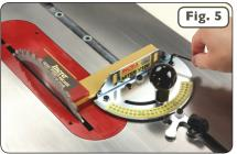
your table top can also be made by loosening the same fasteners and placing a paper shim between the bracket and the underside of the protractor.
