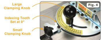
S Using the supplied 1/8" hex key, loosen the (4) button head fasteners that secure the faceplate to the protractor and, depending on your application, square the faceplate to the blade, miter slot, sanding belt, etc. **NOTE:** When squaring to a saw blade (see Figure 5), use a reliable square for this important alignment. Securely retighten the (4) button head fasteners to complete the alignment.
