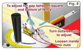
bracket as shown in **Figure 8**, and then tighten the other outside nut by the same amount in the same direction against the rear leg. Alternate this 1/6 turn procedure between the two nuts until the fence is perfectly square to the table DO NOT TURN THE SET SCREW and DO NOT over tighten the nuts. It usually takes less than 1 full turn of the nuts to square your fence to the table.
