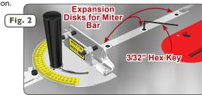
Remove the large clamping knob and disengage the indexing tooth from the protractor. Pivot the protractor head to access and adjust the fourth expansion point. See Figure 3. Replace the large clamping knob and washer.
