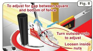
the bracket as shown in **Figure 8**, and then tighten the other outside nut by the same amount in the same direction against the rear leg. Alternate this 1/6 turn procedure between the two nuts until the fence is perfectly square to the table DO NOT TURN THE SET SCREW and DO NOT over tighten the nuts. It usually takes less than 1 full turn of the nuts to square your fence to the table.
