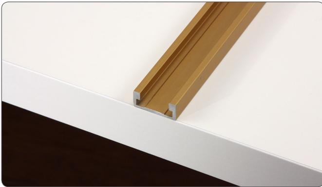
As an alternative, you can drill and countersink mounting holes in your INCRA Miter Channel and mount to your application using #8 flat head screws. Drill the holes with a .219" diameter standard twist drill bit then countersink to a depth that brings the top of the fastener head just below the surface of the extrusion.
