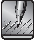
To mark with a 0.5mm Mechanical Pencil: Just hold the pencil vertically and draw a short line in one of the slots, or twist the pencil in a hole to mark a dot.
