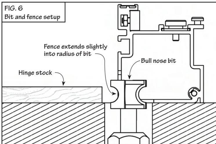
Place the end grain of the hinge blank against the fence and, using a good rubber soled push block, move the stock through the cut. Repeat the cut on the opposite end of the stock, **Fig. 7**. The bull nose cuts should always be made *across* the grain as shown. Attempting to produce hinges with the bull nose cuts made parallel to the grain will result in hinge knuckles that splinter and break easily.
