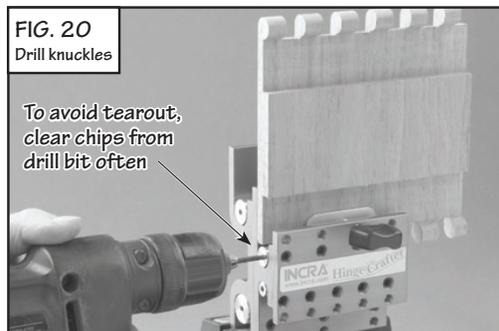
For extra long hinges, first drill one end of the hinge blank, then unclamp, reposition and drill the opposite end of the hinge blank. Finally, unclamp and reposition with the center of the hinge in the HingeCrafter and drill through the existing outer holes to reach the center. For the longest hinges it will be necessary to complete the holes in the center by drilling from both ends and in a few cases a third repositioning is required, **Fig. 21**.
