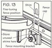
RIGHT of 90° add shims to RIGHT of the miter assembly to increase the angle In general, to raise any miter setting to one of the fractions of a degree shown on the chart, add the required shims:
