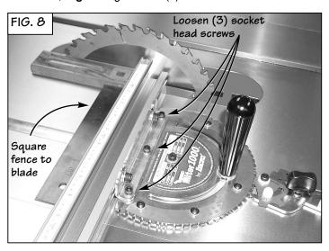
This one-time calibration prepares your INCRA Miter 1000 for work in either miter slot. Just remember that the accuracy of the INCRA Miter 1000 at any subsequent setting is dependent upon the accuracy of your initial 90° calibration. Verify this calibration with a test cut and fine-tune as necessary.
