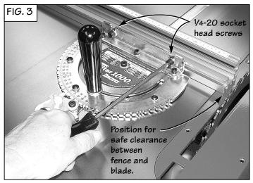
Using the (2) #10-32 x 1/2" thumbscrews with washers and hex nuts, slide the stop positioner into the T-slot located on the front face of the fence.
