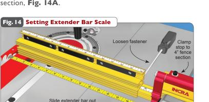
until flip arm is 16" from blade then tighten fastener
