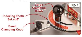
2 Using the supplied 1/8" hex key, loosen the (4) button head fasteners that secure the faceplate to the protractor, and depending on your application, square the faceplate to the blade, miter slot, sanding belt, etc. **NOTE:** When squaring to a saw blade (see **Figure 5**), use a reliable square for this important alignment. Securely retighten the (4) button head fasteners to complete the alignment.
