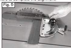
This important one-time adjustment prepares your INCRA Miter V27 for perfect angles at all other indexing tooth positions. Verify the accuracy of your alignment with a test cut, and re-align if the cut is not exactly 90 degrees.
