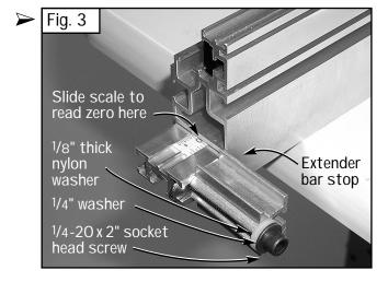
When not in use, the extender bar and stop can be stored in the fence. Just slide the extender bar out, turn it over so that the scale is face down, and insert back into the fence. Tighten the fastener to secure the bar, **Fig. 4**.
