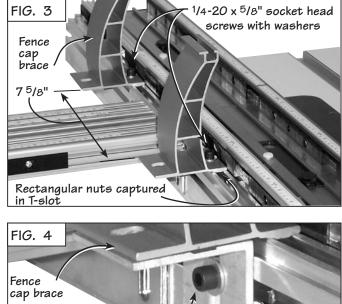
rence cap brace 1/4-20 x 1/2 socket head screw with washer Support bracket rectangular nut captured in T-slot
