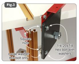
on the remaining  $1/4-20 \times 7/8$ " hex bolt and insert through the hole on the side panel. Add a split lockwasher and a square nut then tighten the assembly in place, **Fig. 5**.
