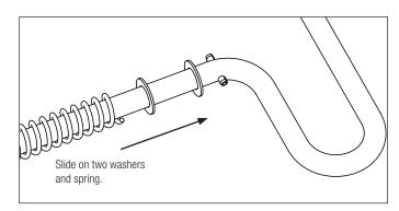
**STEP 1:** Slide on the two washers and the spring as shown.
