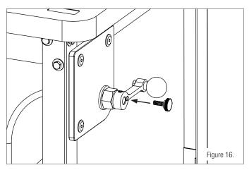
**Figure 16**. Now thread the brake knob into the threaded hole in the handle. Do not tighten the brake knob until it's needed. Use this when heavy routing is planned.
