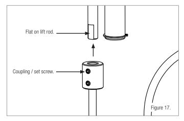
Figure 17. Attach the remaining coupling on the other end of the flex shaft and then to the lift rod. Make sure to align the set screw with the flat on the rod before tightening the screw. Use the crank handle to turn the flex shaft and coupling. If you need to turn the lift rod, keep your hands clear while using the lift wrench to lower the motor to the bottom end of its travel. Keep the wrench engaged which will take the pressure off the lift rod making it easy to turn by hand.
