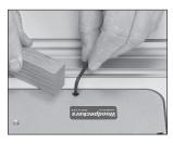
the plate feels flush, use a block of wood to make sure it doesn't catch going either direction then adjust the remaining screws.
