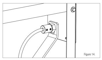
**Figure 14**. Apply a dab of grease on the outside of the pin and insert it through the hole in the side panel bolt. **This will take some effort.** Be careful not to kink the flex shaft. Bend it just enough to get the pin through the hole.
