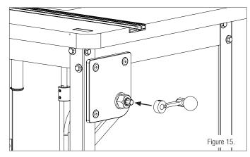
Figure 15. From the outside, slip the crank handle onto the pin, align the end of the pin with the face of the handle, align the set screw with the flat spot on the pin and tighten the screw.
