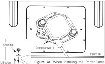
7518, there is only one way it can go in. Before inserting the motor make sure that all four clamp screws are loose. Orient the motor in whatever orientation is necessary for it to go all the way
