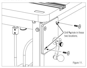
Figure 11. Using the side panel as a guide, drill two %2 dia. holes through the router table stand. Fasten the panel in place using the remaining connector bolts and nuts.
